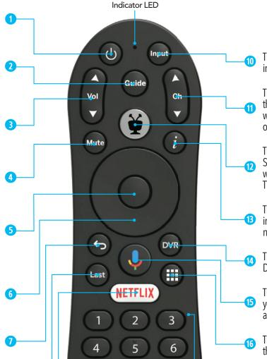
The Input Button changes inputs on the TV.
